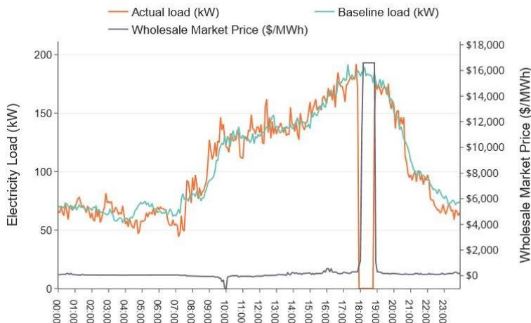
While this can be an effective method of estimating customer loads during events, as shown in the example, there are certain cases where this algorithm is not entirely effective. Most commonly this occurs for sites with highly variable or intermittent loads, such as the example below of a pumping site:
