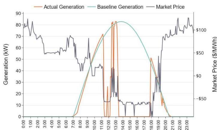
In this example, the baseline algorithm can produce a generation estimate that approximates the expected generation quite strongly. We can then identify the periods where ramp-down has been implemented by the kWatch controller, for which the wholesale market price is below a designated, site-specific price threshold.
