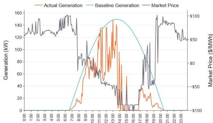
In this example, there is significant variability in the generation output, which causes the baseline to be a much weaker approximation of expected generation. Unfortunately, without extensive additional metering of local weather data and irradiance levels, it is nearly impossible to produce a strong approximation of generation curves subject to shading.
