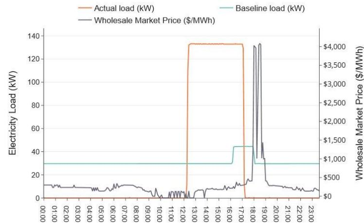
In this example, due to the variability of the load, the calculated baseline shows a result that does not reflect the expected usage of the site during the event period, which is clearly higher than estimated.
